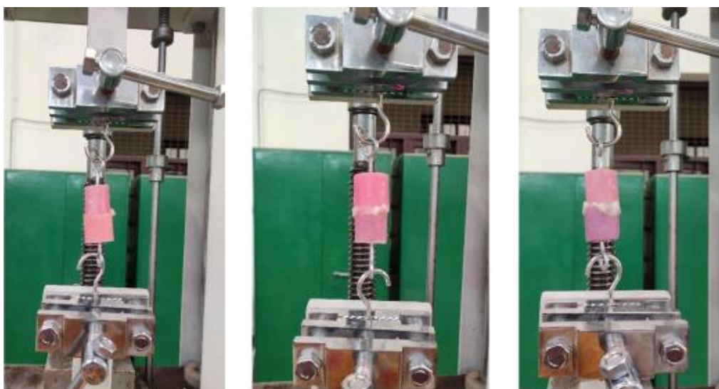
Fig. 6. Test cylinders coated with Fittydent positioned in the Instron machine.
