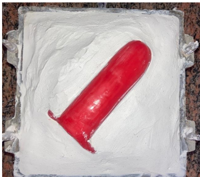
Fig. 3. Wax pattern invested in a flask.
