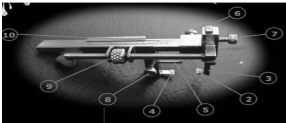
Fig. 3. DT3C Device. (1) Lingual arm. (2) Lingual arrow blade. (3) Labial arm. (4) Labial arm blade. (5) Vertical stop. (6) depth lock. (7) Lingual arm lock. (8) vertical stop lock. (9) Guiding screw & nut. (10) Horizontal scale.
