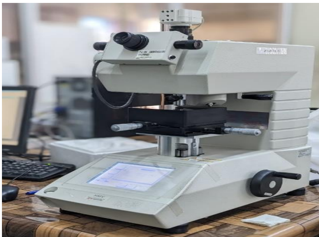
Fig. 14. Vickers Microhardness tester for measuring microhardness of cured resin cement.
