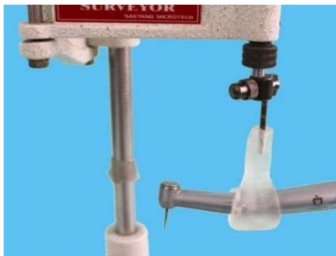
Fig. 1. The handpiece is attached to the surveyor using a custom-made device.
